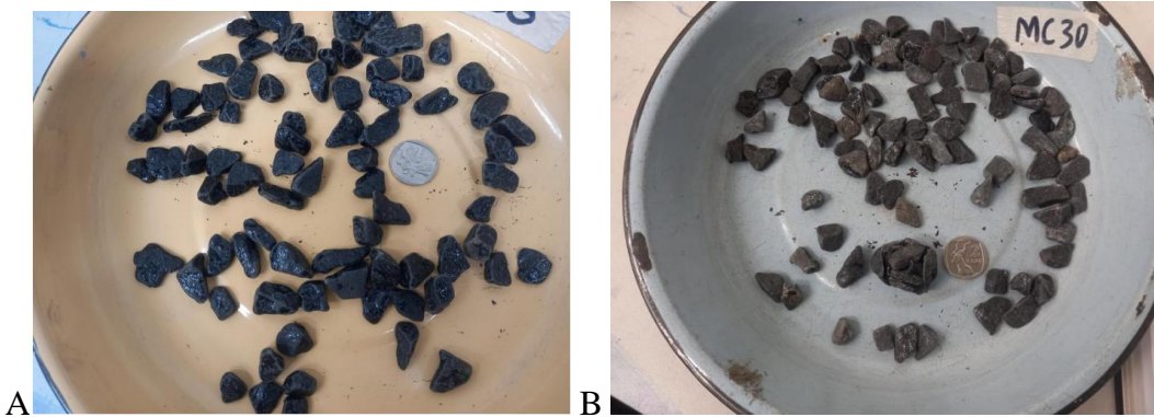
Figure 7: Visual Investigation of the adhesion of the prime products: A. C55 Emulsion Prime and B. MC30 Cut-Back Bitumen Prime.
