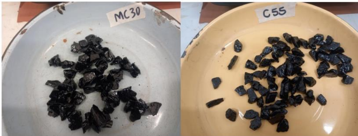
Figure 5: The coated aggregates before rolling bottle test
