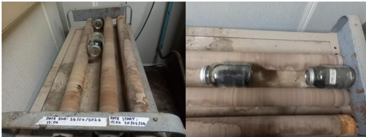
Figure 6: Rolling Bottle test with the C55 and MC30 Prime subjected to the mechanical rolling machine
