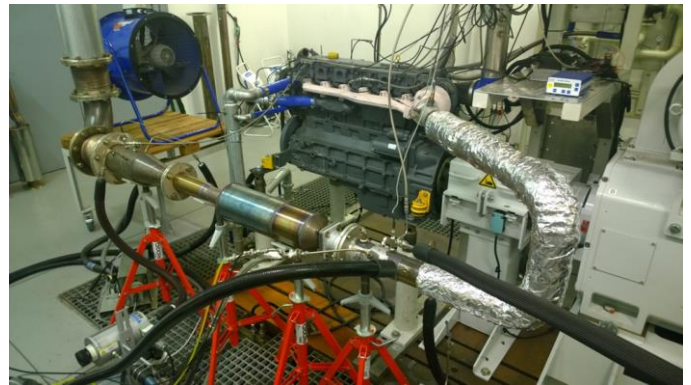
Figure 2. Deutz BF 6M 1013 E engine in a test cell at the Sasol Fuels Application Centre.
