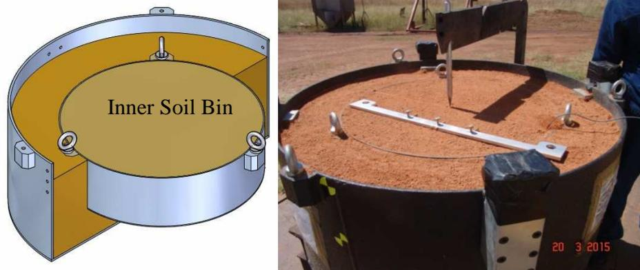
**Figure 2: Soil ejecta test set-up**
