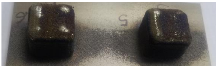
Figure 2: LENS fabricated TiAl coupons by method of in-situ alloying.
