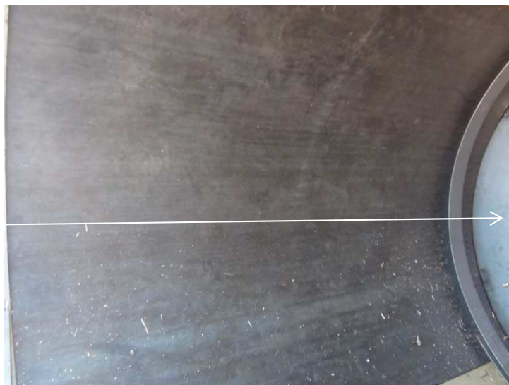
Figure 13: Exposed surface of conveyor belt material to fragments and blast, along the length of the chamber.
