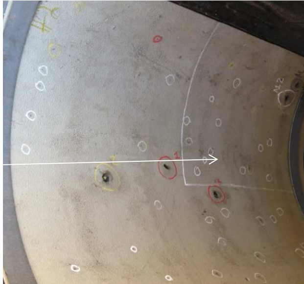
Figure 18: Exposed surface of Polyurea material to fragments and blast, along the length of the chamber.
