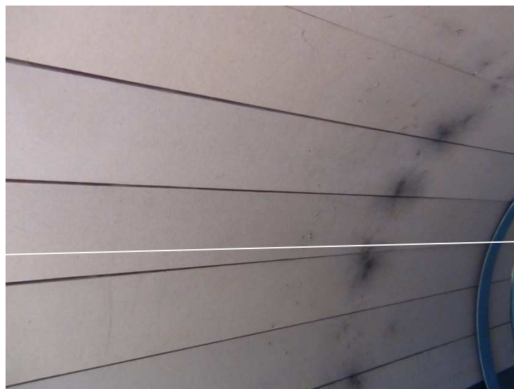
Figure 15: Exposed surface of Supawood material to fragments and blast, along the length of the chamber
