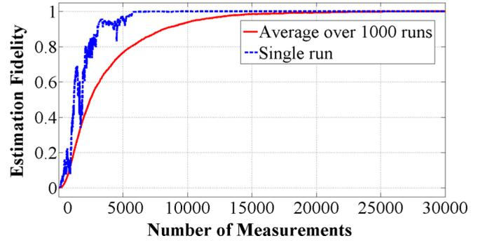
FIG. 2. (Color online) Estimation of the Larmor frequency and axis of rotation for a spin- $\frac{1}{2}$  particle. The estimation fidelity for the probability distribution of the dynamical parameters as a function of the number of measurements for a single run (dashed blue line) and averaged over 1000 runs (red line).
