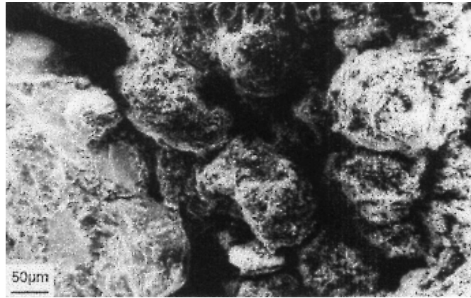
Fig. 33. Scanning electron micrograph showing evidence of inadequate braze processing.
