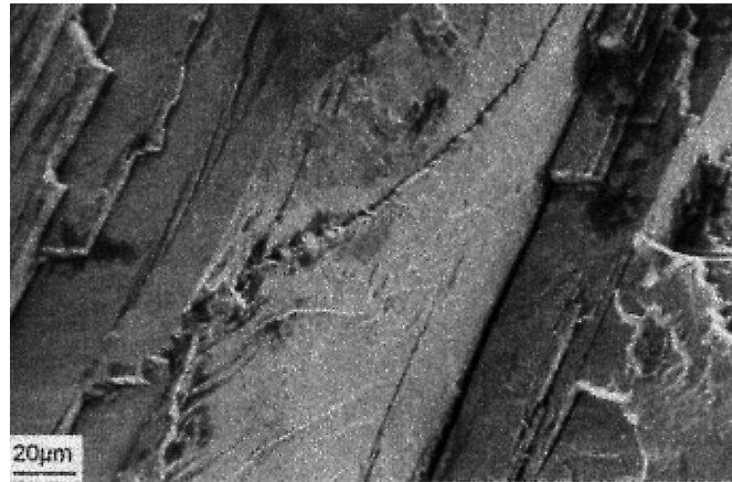
Fig. 30. Scanning electron micrograph of the fracture surface of the braze material at \Delta K \approx 16 \text{ MPa} \sqrt{\text{m}} .
