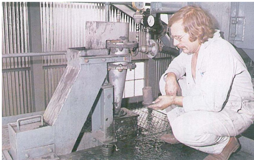
Figure 4. 150 mm cyclone in FRI dense-medium fine coal pilot plant
