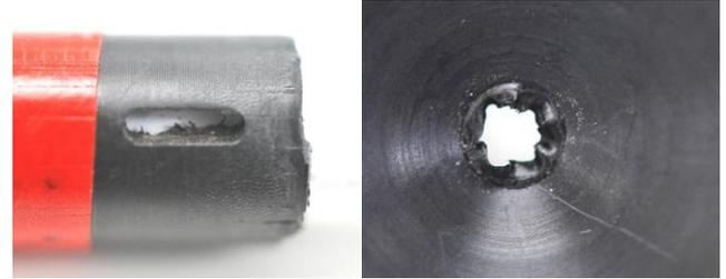
Figure 1. Burrs in the inlet aperture (left) and in the outlet aperture (right) of an X-Sampler
