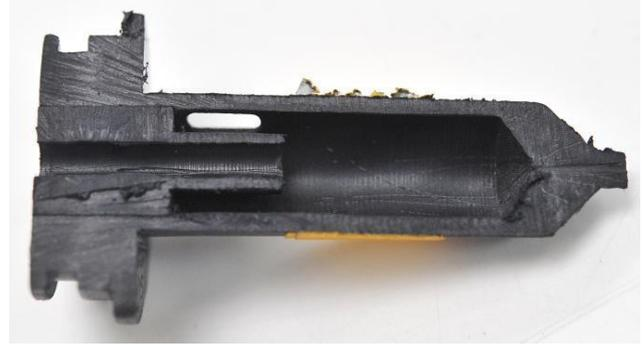
Figure 5. Inside view of a Y-Sampler
