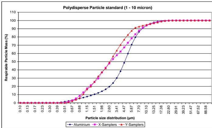
Figure 6. PSD of filters where PPS test dust was sampled
