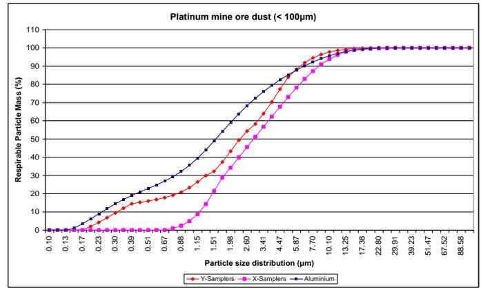
Figure 8. PSD of filters where platinum mine ore dust was sampled
