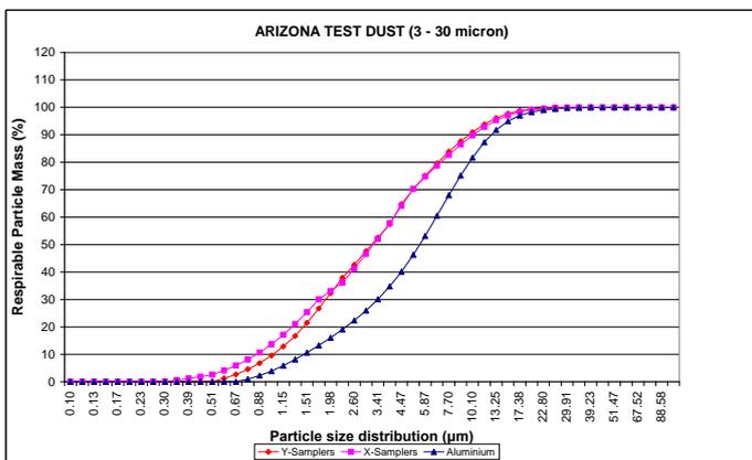
Figure 7. PSD of filters where Arizona test (3 – 30  $\mu\text{m}$ ) dust was sampled
