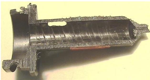
Figure 4. Rough inside surface of an X-Sampler
