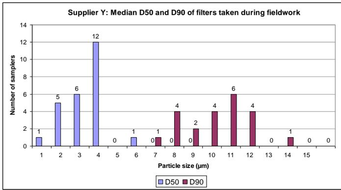
Figure 10. Median D50 and D90 values obtained from the Y-Samplers after real sampling at three platinum mines
