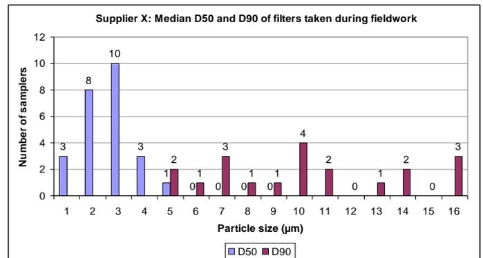
Figure 9. Median D50 and D90 values obtained from the X-Samplers after real sampling at three platinum mines
