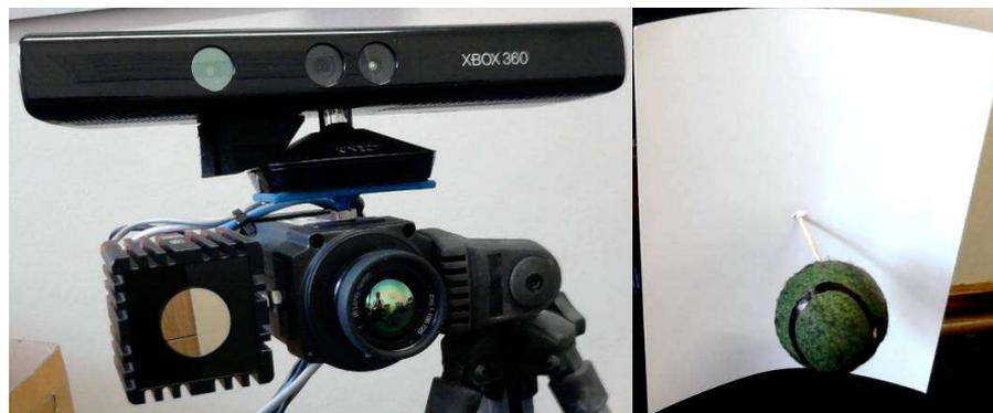
*Figure 7: Multi-sensor setup with SR4000 TOF camera, FLIR A300 IR camera and XBOX Kinect rigidly mounted on a tripod (left), and tennis ball calibration object(right).*
