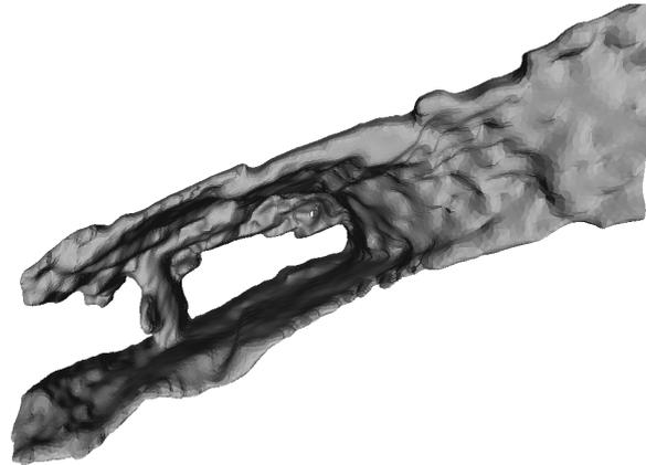
*Figure 5. SR4000 data visualisation using a ray carving technique.(Gold Reef City Mine)*
