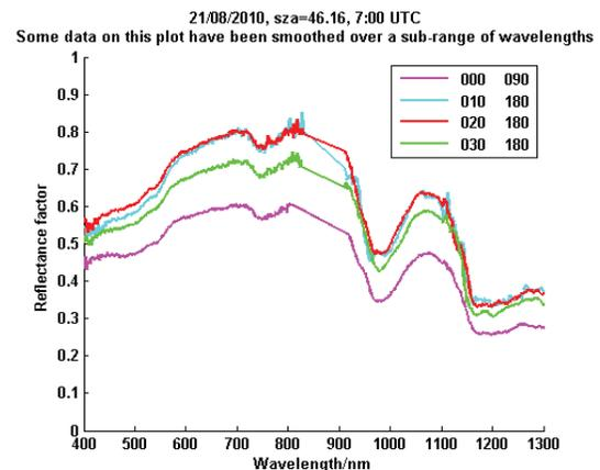
Figure 4: Tuz Gölü BRDF measurements the surface structure of the salt flat.
