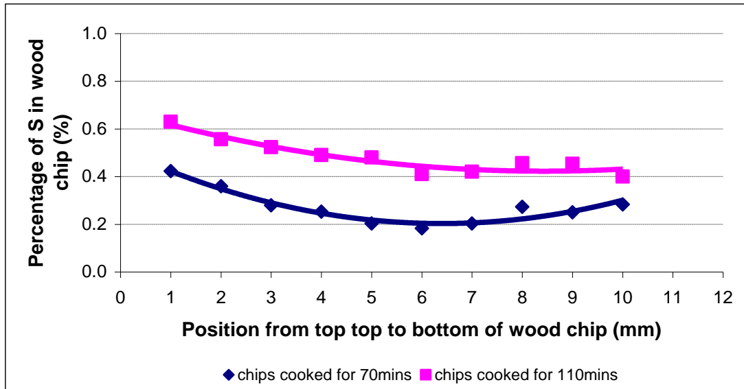
Figure 9. Average sulphur content for three chips cooked for 70 and 110 minutes measured using ESEM/EDX.
