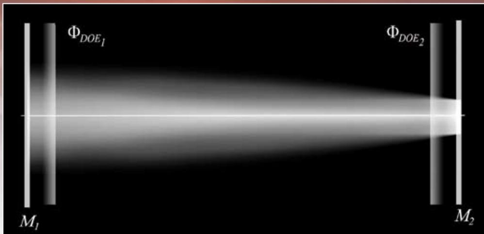
The resonator concept, as shown here, comprises two transparent DOEs (like lenses) at either end as well as the usual bounding mirrors to complete the box.
