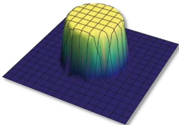
A fat-top profile laser beam; such beams have a constant energy density in the central part of the beam, that sharply falls to zero at the edges.
