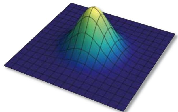
A Gaussian profile laser beam, with a characteristic peak at the centre and slow decay at the edges.
