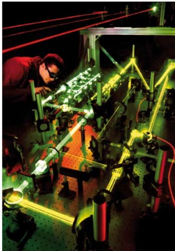
A technician evaluates the interaction of multiple lasers that will be used aboard the Airborne Laser. Image: Wikimedia commons
