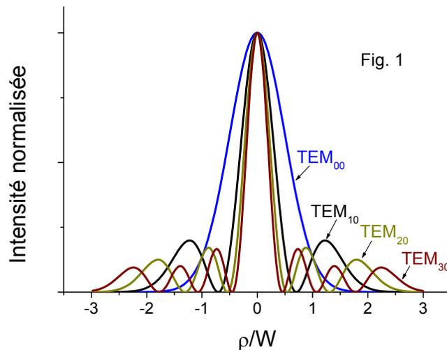
Figure 1. Radial intensity distribution of the four-first symmetrical Laguerre-Gauss TEM<sub>p0</sub> beams.
