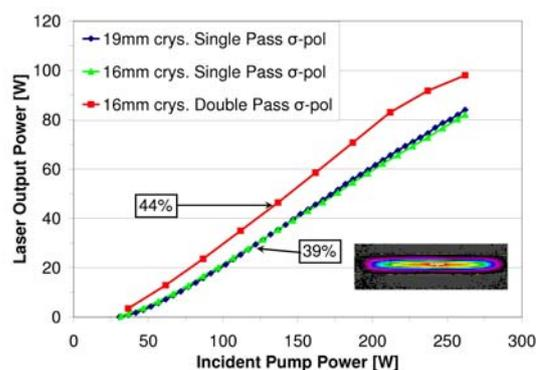
Fig. 2: Output powers of various Tm:YLF slab lasers.
