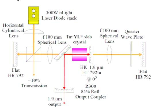
Fig. 1: Experimental setup of the multi pump pass slab laser
