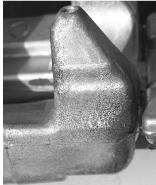
FIGURE 5: An example of the rough surface finish of a lubricant defect brake caliper casting produced during trials with the CSIR-RCS-HPDC cell.
