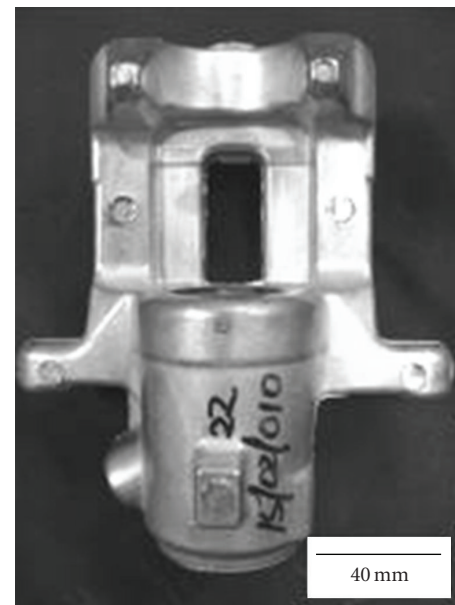
FIGURE 1: Example of the rheocast aluminum brake caliper including the runner and the biscuit in part drawing (a) and the actual premachined component (b).
