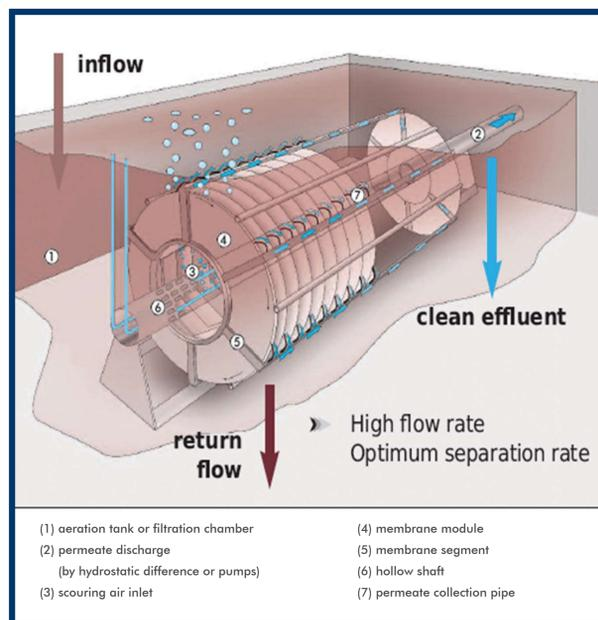
Figure 1: MBR system that could be applied in the IRIP concept
