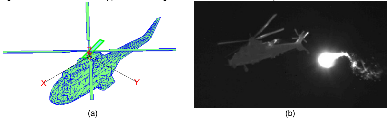
Figure 8: Aircraft modelled by polygons, and a real-world flare dispensing
