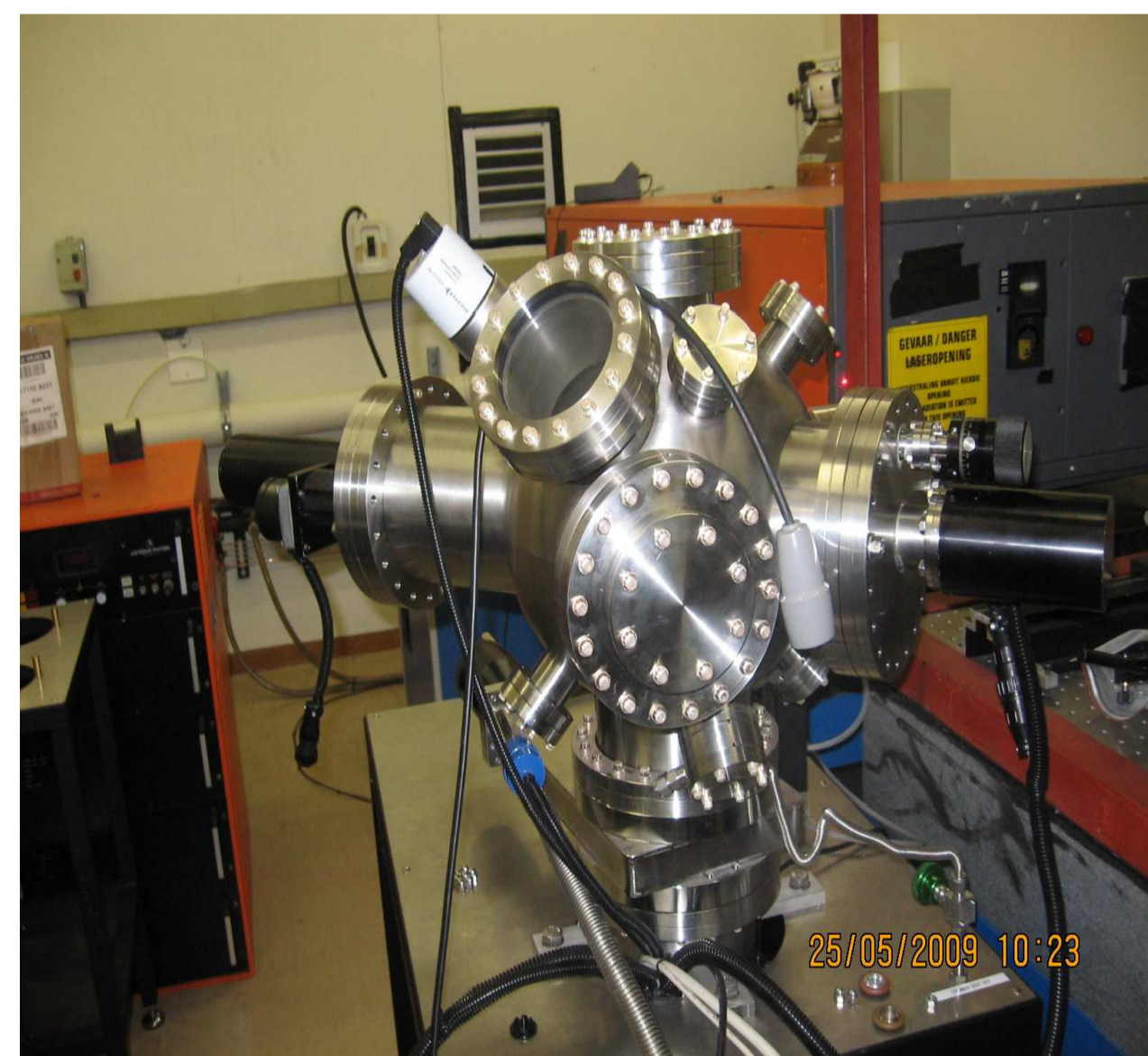
The Pulsed laser deposition system showing the deposition chamber and the observation window
