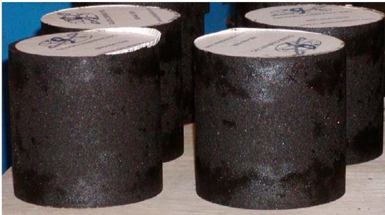
Figure 1. Gyratory compacted oil sand specimens.
