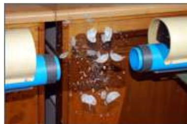
The hail gun releasing hail stones, targeted to hit the heliostat mirror panel
