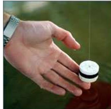
Keofloats allow researchers to determine small wave sizes accurately in a specific harbour layout
