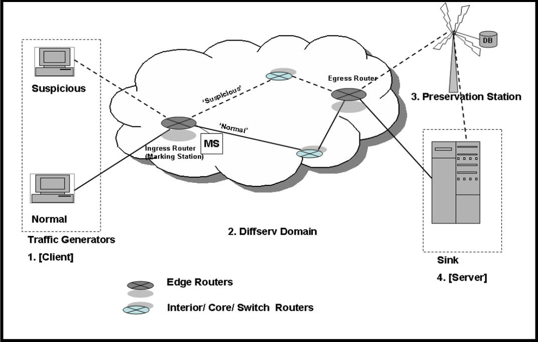
**Fig. 1: The Conceptual view of the Logical Traffic Isolation Using DiffServ**
