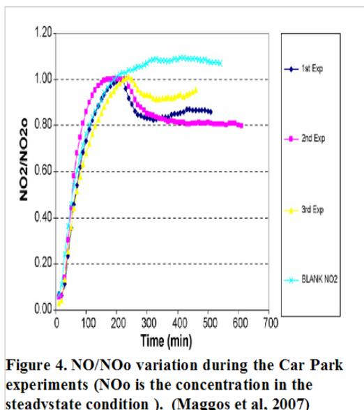
Figure 4. NO/NO<sub>o</sub> variation during the Car Park experiments (NO<sub>o</sub> is the concentration in the steadystate condition). (Maggos et al, 2007)
