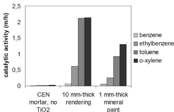
**Figure 2. Photocatalytic activity of the cement-based materials at 300 ng/LBTEX nominal concentration, PICADA Results. (Vallee, F, et al ,2004)**
