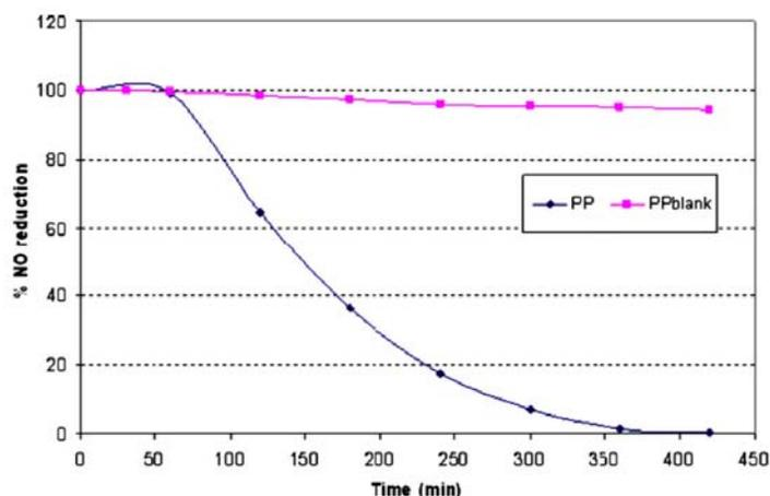
Figure 5. Percentage of NO removal during laboratory scale experiments. (Maggos et al, 2007)
