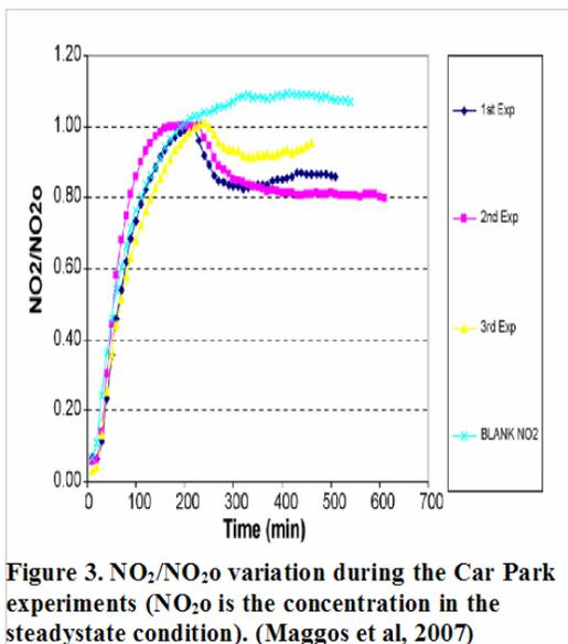
Figure 3. NO<sub>2</sub>/NO<sub>2o</sub> variation during the Car Park experiments (NO<sub>2o</sub> is the concentration in the steadystate condition). (Maggos et al, 2007)
