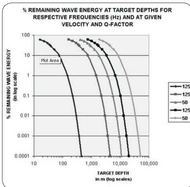
Fig. 4: Penetration depths as calculated by the spreadsheet.
