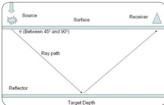
Fig. 1: Schematic diagram of the seismic data acquisition process.
