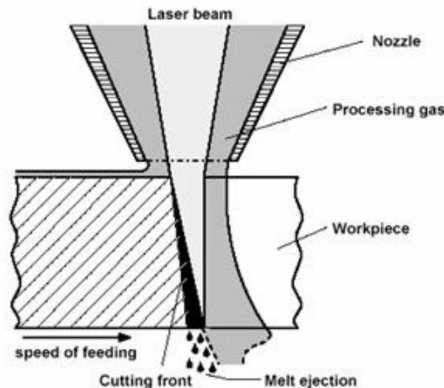
**Figure 1 Diagram of the laser cutting process.**
