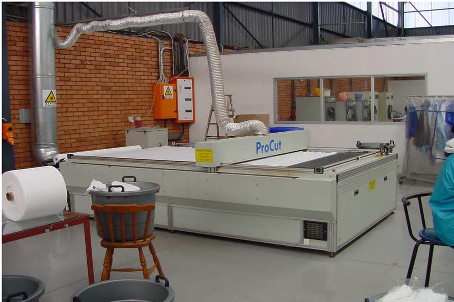
**Figure 4 ProCut Laser cutting system at Tappo Industries**
