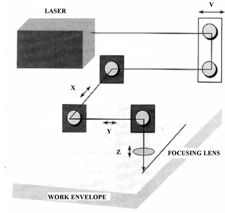
Figure 3 Diagram of "flying optics" beam delivery.
