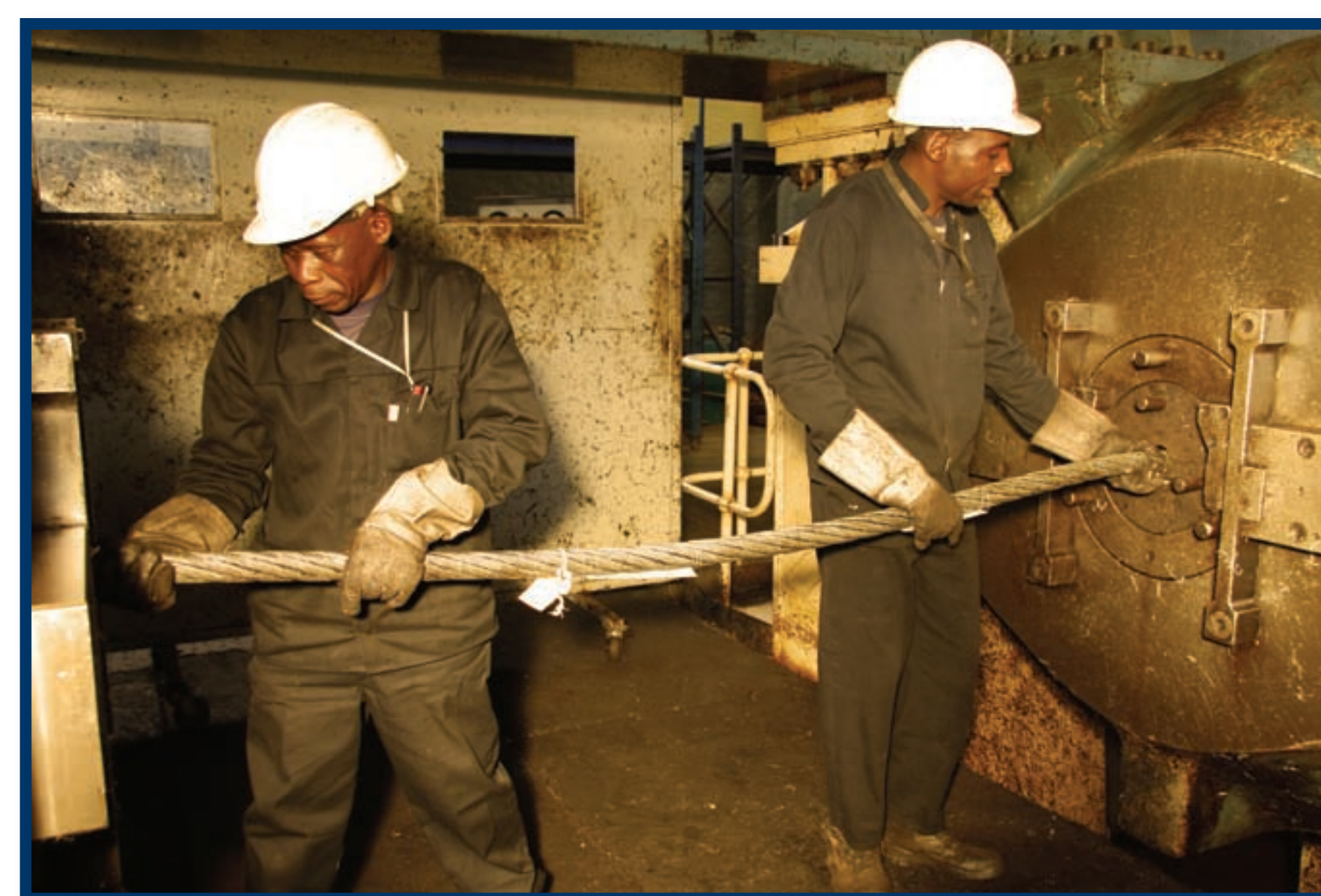
CSIR staff inserting a rope specimen between the cross-heads of the 15MN tensile test machine
