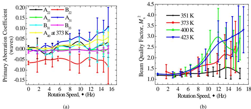
Fig. 7. (a) Higher order aberrations introduced by the SPGL; (b) increase in  $M_x^2$  with rotation speed and temperature as a direct result of the aberrations in (a).
