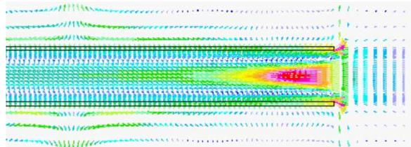
Fig. 1. A cross-section of a SPGL showing the velocity distribution of the gases as the warmer gas near the wall escapes, and is replaced by the cool air which enters along the axis. (Fig 1 Movie [5.3 MB])
