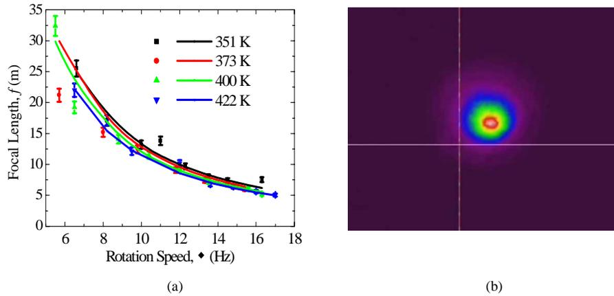
Fig. 4. (a) The focal length of the SPGL as calculated from the optical wavefront and confirmed by inspection, and (b) the intensity distribution during rotation ( $T = 422$  K). (Fig 4b Movie [0.15 MB])
