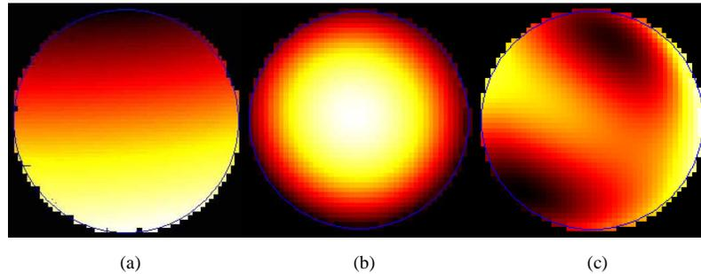
Fig. 6. The phase distribution of the laser beam with: (a) no rotation but heated to 422 K, showing tilt; (b) after rotating the SPGL at 17 Hz, showing significant curvature on the wavefront; and (c) same conditions as in (b) but with defocus and tilt removed, revealing the higher order aberrations.
