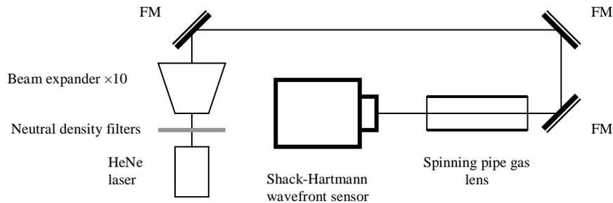
Fig. 3. Experimental set-up. (FM = Flat mirror).
