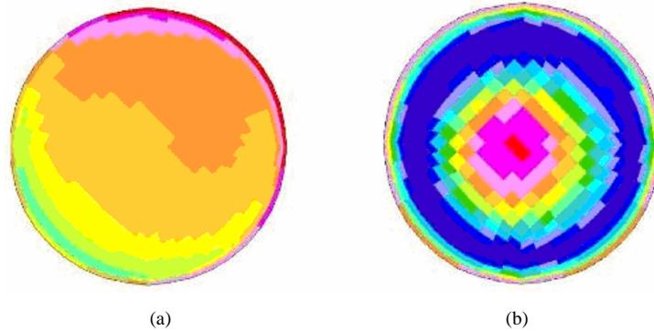
Fig. 2. Cross-sectional density profiles of an SPGL showing: (a) the initial state after heating, and (b) the rotating steady-state near the end face of the pipe, with high density centre (red) and low density edges (blue). (Fig 2 Movie [4 MB])
