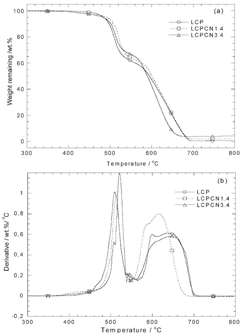
Figure 15. a) TGA thermograms and b) first derivative TGA (DTGA) curves of neat LCP and its nanocomposites under air atmosphere.
