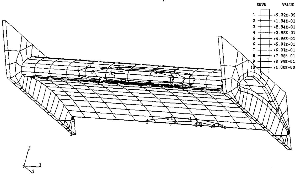
Fig. 5. Contour plot of total damage parameter  $w_{tot}$ .
