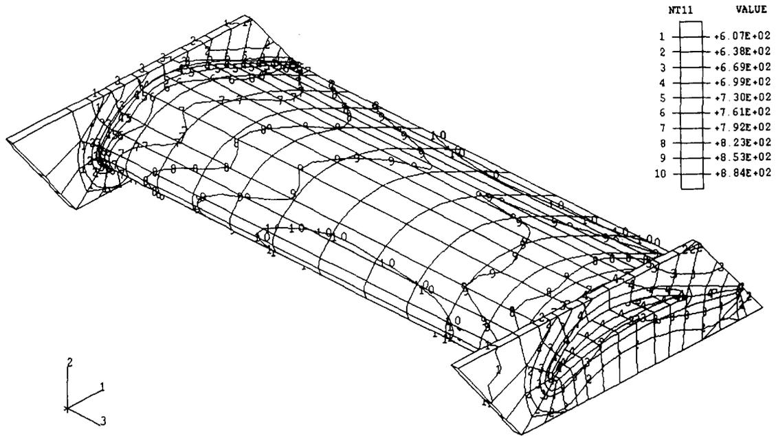
Fig. 1. Blade metal temperature distribution.
