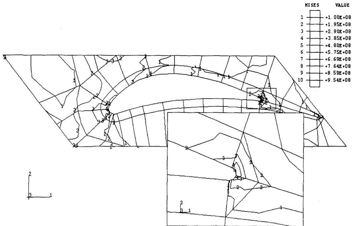
Fig. 2. Von Mises stress distribution.
