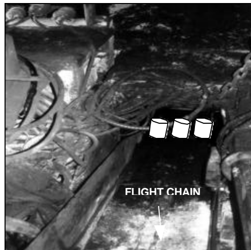
Figure 3.2.11: Position of the air movers in the throat of the flight conveyor
