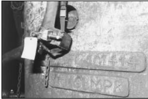
Figure 2.2.1d: Position of samplers at the operator's position (mine sample)
