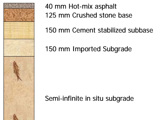
Figure 7. The pavement structure used for modelling purposes
