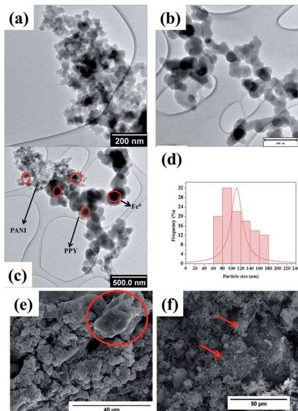
Fig. 2 TEM images of (a)  $\text{Fe}^0$ -PANI, (b)  $\text{Fe}^0$ -PPY, (c)  $\text{Fe}^0$ -PPY/PANI (d) particle size distribution of  $\text{Fe}^0$  nanoparticles in  $\text{Fe}^0$ -PPY/PANI and SEM image of (e) PPY/PANI and (f)  $\text{Fe}^0$ -PPY/PANI.
