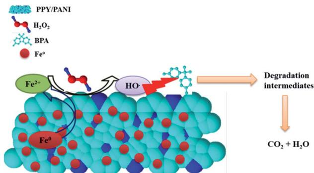
Fig. 13 Advanced Fenton reaction mechanism for the degradation of BPA using Fe<sup>0</sup>-PPY/PANI.
