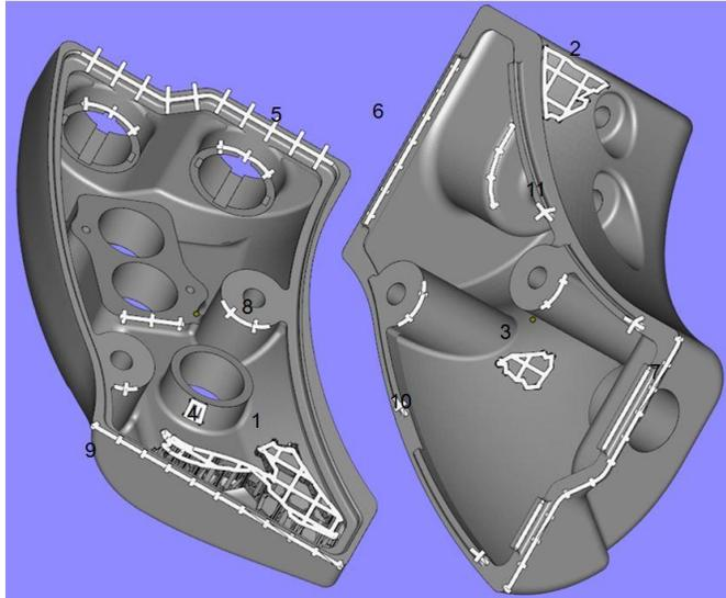
**Figure 5: Support structures for first test build**
