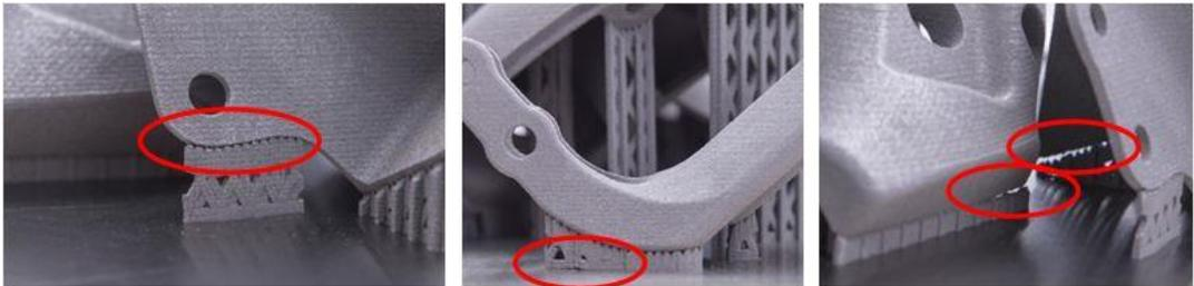
**Figure 9: Partially broken support structures**
