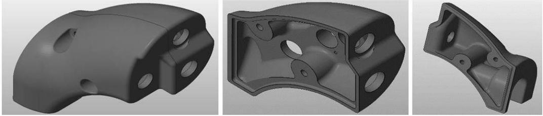
Figure 3: Throttle lever grip
