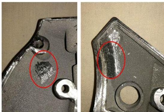
**Figure 11: Areas with difficult support removal**
