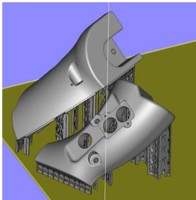
Figure 4: Build layout of the throttle lever grip parts
