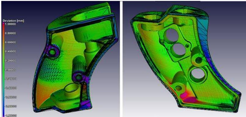
Figure 12: Comparison of microCT to CAD
