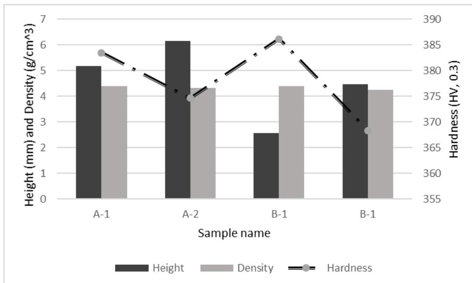
Figure 2: Microhardness variation, Density and Height measurements of the samples fabricated at different processing conditions.
