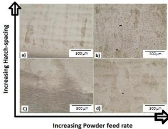
Figure 1: OM micrographs of Ti-6Al-4V by LENS at different process conditions a) B-1, b) B-2 c) A-1 and d) A-2
