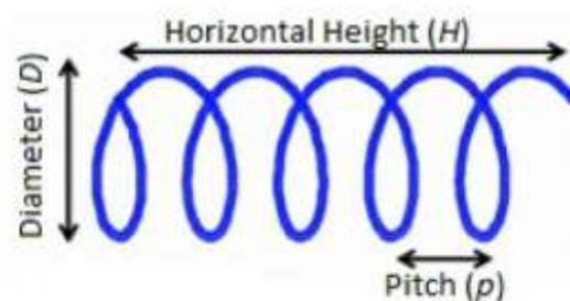
Figure 3: Geometry of a spiral (Lutchman 2018)
