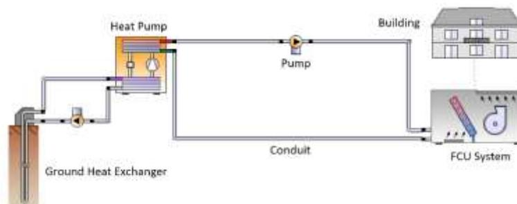
Figure 3: Layout of geothermal heat exchanger with a heat pump system (Lutchman 2018)
