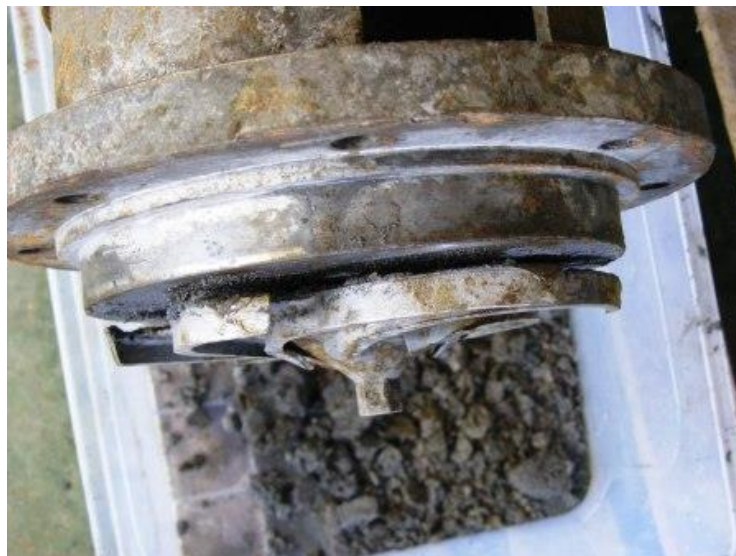
Figure 5. Single vane pump impeller with Ti metal powder visible behind the back plate.
