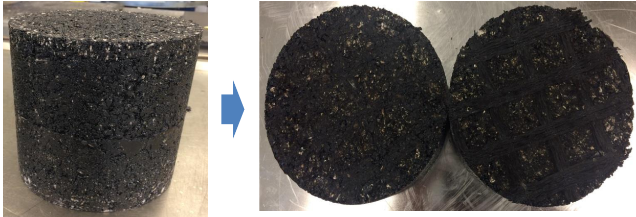
1 2 FIGURE 6 Example HMA Sample Failure Mode (FA-50 Reinforced).
