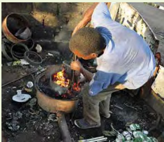
Melting the aluminium waste Photo credit: © Afrique in visu
