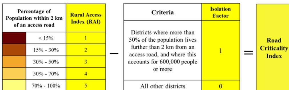
Figure 5. Calculation and parameterisation of road criticality index
