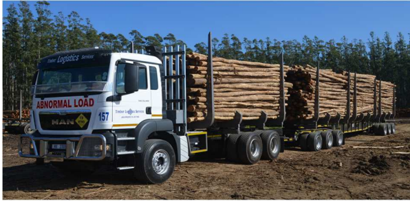
Fig. 5a 27.67 m, 73.5 t rigid-drawbar. Payload = 52.14 t
