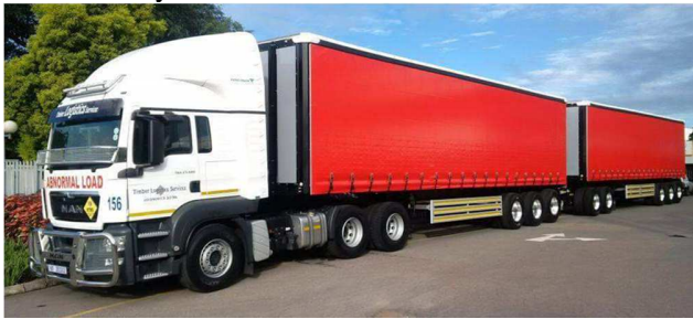
Fig. 5c 29.6 m, 83.8 t A-double. Payload = 53.4 t
