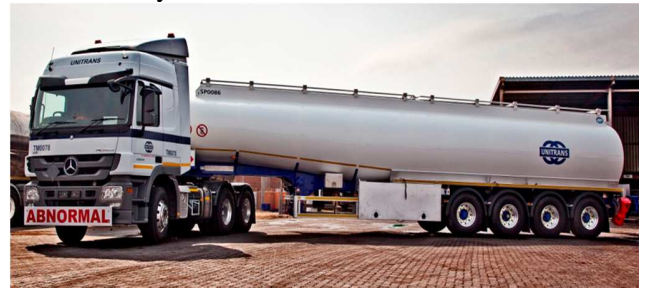
Fig. 5d 18.6 m, 57.7 t TT/quad semi-trailer. Payload = 55 000 ℓ (40.2 t)
