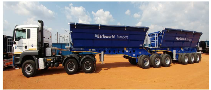
Fig. 5b 21.6 m, 73.7 t B-double side-tipper Payload = 50.55 t
