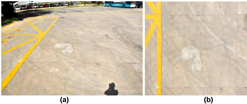
Figure 7: Image warping: (a) original image, (b) birds-eye view image after warping
