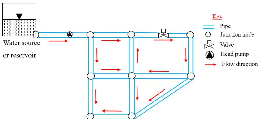
**Figure 2:** Schematics of a water distribution network.
