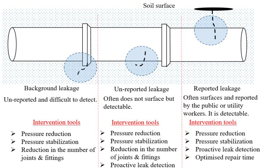
Figure 5: Leakage types and intervention tools [23].
