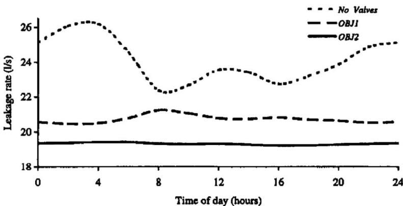
**Figure 4:** Leakage flow rate comparison with and without pressure regulating valves [22].
