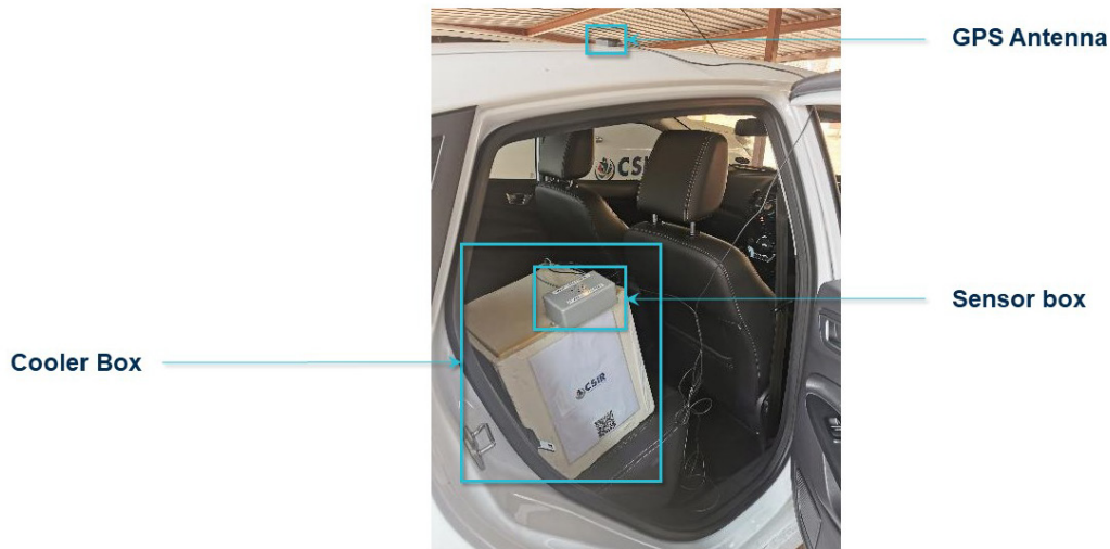
Figure 3: Illustration of the cold chain track and trace sensor box and a polystyrene cooler box in the backseat of the car, during the field testing of our implementation. A temperature and GPS antenna are attached to the sensor box. (Source: Authors)
