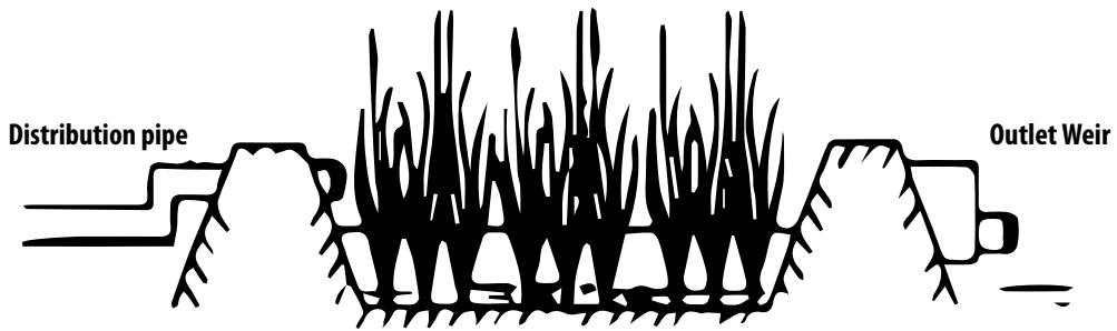
Figure 3.2: Horizontal free water surface (Source: Vymazal et al. , 1998, Kadlec and Wallace, 2008)
