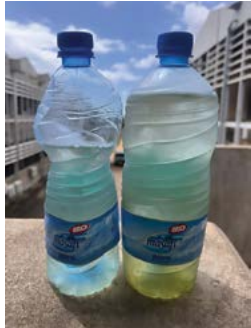
Figure 8.2: Effluent of the constructed wetland for visual appearance (Credit: Leah Marwa, 2023)
