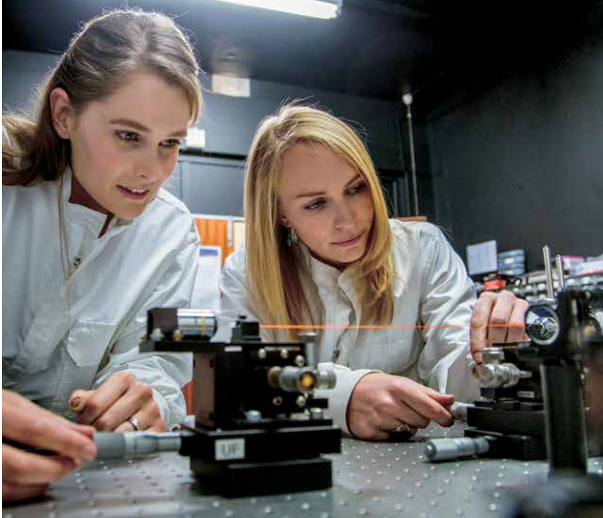
Dr Angela Dudley (left) and Melanie McLaren in the laser laboratory, where Dr Dudley uses digital holograms to measure the fundamental properties of light. While there are many commercial devices to measure the particular properties of optical fields emerging from lasers and optical fibres, none are able to provide full information on the field. CSIR researchers have used rewritable liquid crystal technology to demonstrate the potential for an all-in-one diagnostic tool, capable of extracting all the key information. The ability to quantify these properties will allow users to monitor the optical performance of a system in real time, with uses in the fibre-optic industry and in photonics research.
