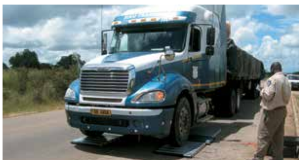
Staff at the Malawi Road Traffic Directorate undertake an axle load survey at Chileka on the road between Lilongwe and Mchinji on the border between Malawi and Zambia.
