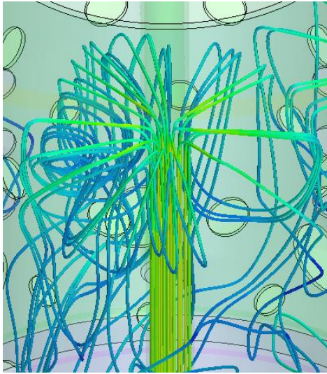
Figure 5: Design E - stream tracers showing a fairly good Rz shape. Score 7/10
