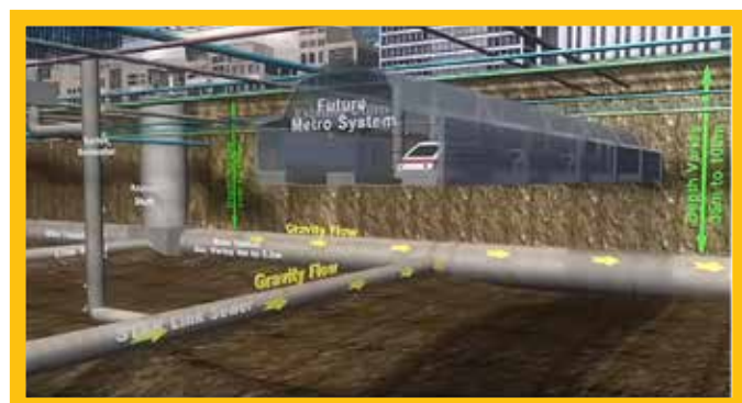
FIGURE 3: Underground view of the deep sewer system
