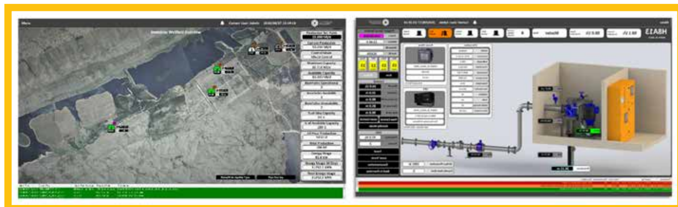
FIGURE 7: Screenshots of SCADA system used to monitor and control the Steenbras Wellfield
