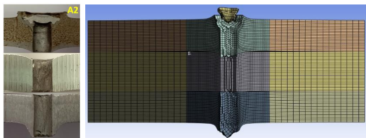
Figure 7: Comparison of plate damage and deformation evident on sectioned plate (A2) versus simulation.
