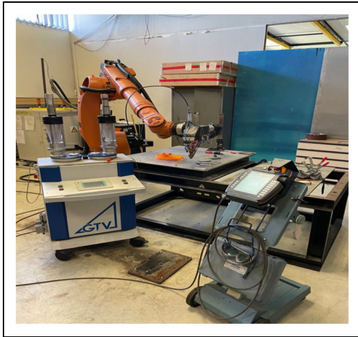
Figure 2. Laser cladding machine at the Council for Scientific and Industrial Research, Pretoria.
